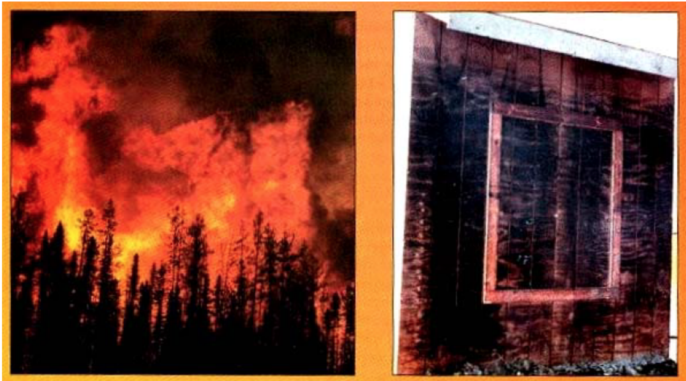
Figure 1. Field experiments demonstrated that radiant heat from a high-intensity forest fire (left pane), which caused substantial scorch, was not sufficient to ignite a vertical wood wall (right pane) located 10 meters (33 feet) away so long as direct flame and ember contact was avoided. Note the lack of wall scorch under the eave because of the radiation "shading" from the eave.
